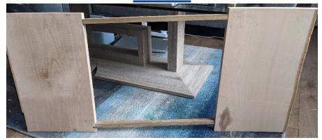
Insert 4 dowels into the ends of the stripwood pieces, then assemble as shown, you can add a little PVA glue into the holes for added security, make sure to wipe away any excess.
