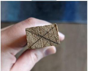
Find the centre point of the stripwood by drawing and X connecting the corners. Drill a hole approximately half the length of your dowels (in our case this would be 15mm) at this centre point.
